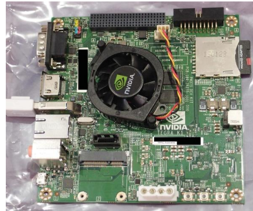
Fig.12: Device used in this experiment (Jetson TK1)
