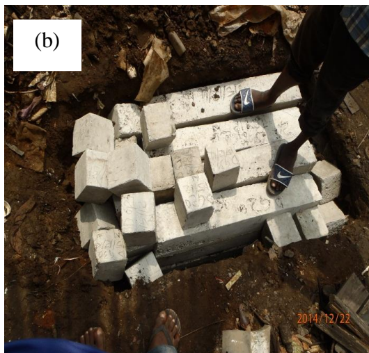
Fig. 3 Placement of concrete specimens in excavated (a) abattoir and (b) hydrocarbon contaminated pits
