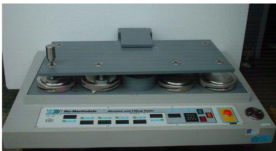
Fig. 3. Abrasion and pilling tester [13].
