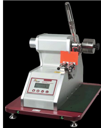
Fig. 4. Elmendorf tearing tester [14].
