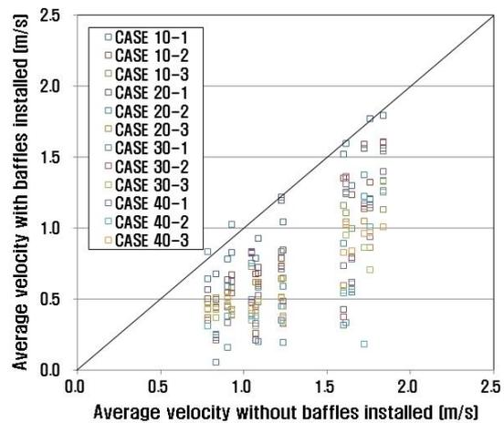
**Figure 7. Comparison of flow velocity measurement data according to baffle installation(B discharge condition)**
