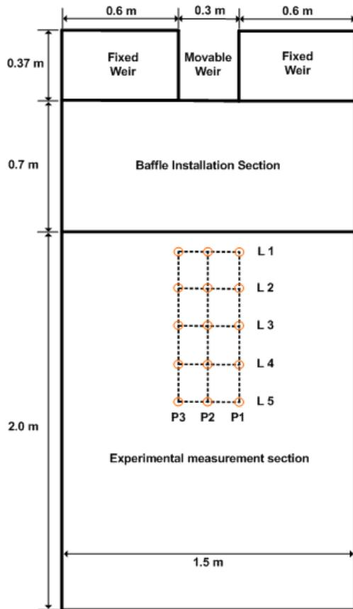
**Figure 4. Baffle installation section**
