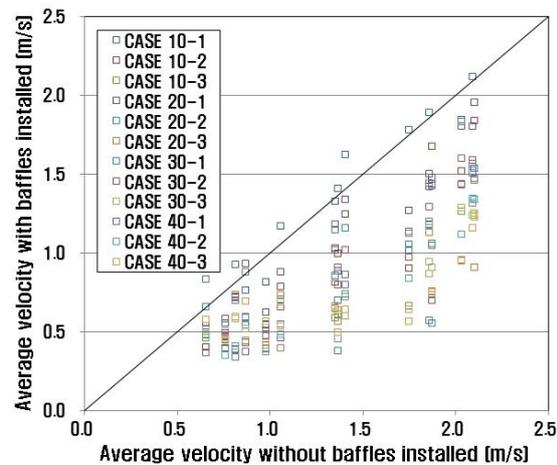
**Figure 8. Comparison of flow velocity measurement data according to baffle installation(C discharge condition)**
