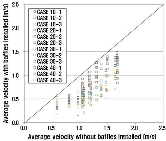
**Figure 6. Comparison of flow velocity measurement data according to baffle installation(A discharge condition)**
