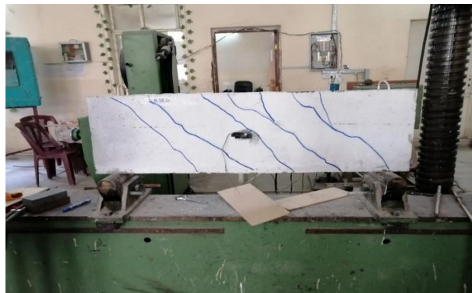
Figure (3). Deformation of the Tested deep Beams
