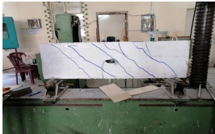
Figure (3). Deformation of the Tested deep Beams
