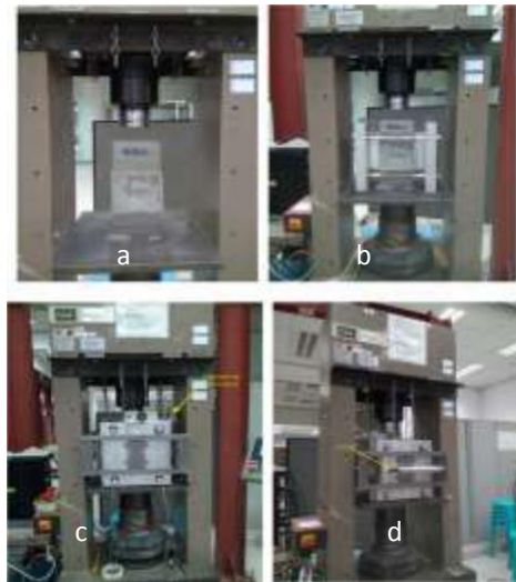
Figure 1: Setup specimen procedure (a) Uniaxial loading, (b) Biaxial loading, (c) Adjustment of plate and (d) Three dimensional setup [2]
