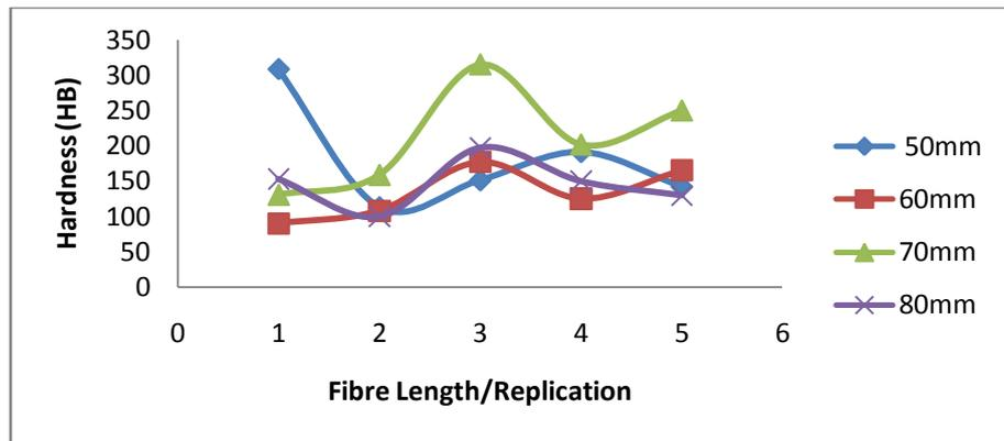
Fig. 2: Graph of hardness at 10%NaOH solution for drying temperature of 50°C
