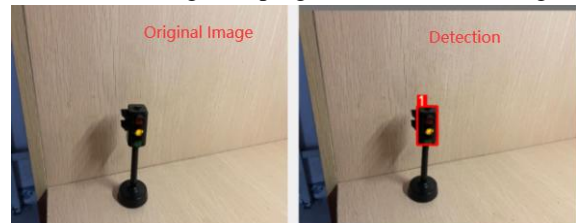
Fig. 8 Identification program yellow light detection
